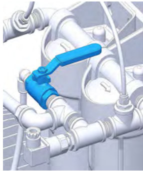
Water valve in closed position
