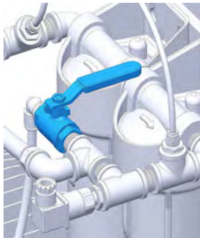
Water valve in closed position
