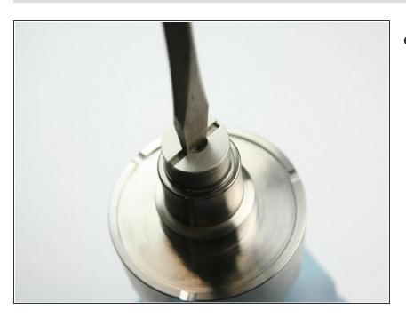
Tighten the poppet retainer into the sealing head body with the flat head screwdriver.
