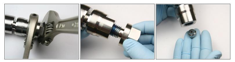
Loosen the <u>high-pressure sealing head gland</u> from the sealing head body with adjustable wrenches.
