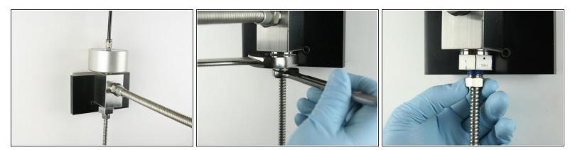
(i) The valve components can be replaced with the <u>valve body</u> mounted to the pump.
