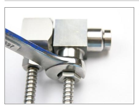
Tighten the high-pressure gland nut into the swivel housing with a 5/8" wrench.
