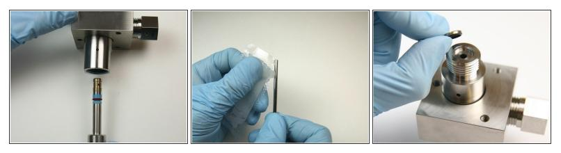
• Put the bleed-down valve tool with the parts into the bottom of the valve body until the tool reaches the bottom of the valve.
