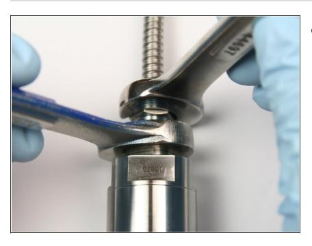
Tighten high-pressure gland into swivel nut with 5/8" and 11/16" wrenches.
